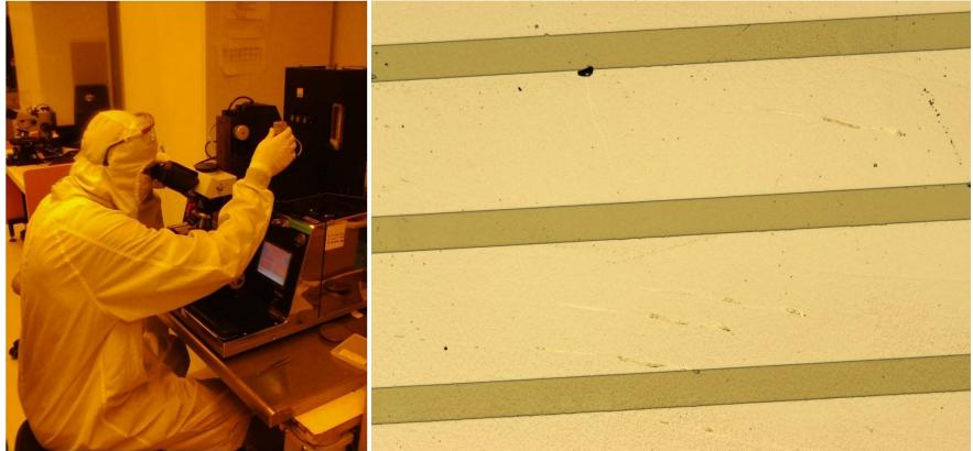
(left) Ph.D. candidate Jeremy Kunz working with the MJB4 mask aligner at the Microelectronics Research Center. (right) Image of 100 µm bars of electron-beam evaporated zinc oxide separated by 400 µm on a GaSb surface. Supported by URC grant (2011): "Transparent Contacts for Dual Optical and Electronic Excitation in Mid-Infrared Semiconductor Lasers" (included training and preliminary work at Microelectronics Research Center, UT-Austin).
