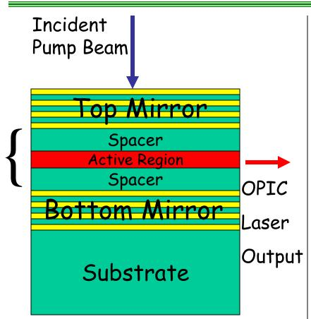
**Principal:** Etalon cavity is tuned to pump  $\lambda$  to bring about several passes through the active region between two distributed Bragg reflectors (DBRs). **Goals**
