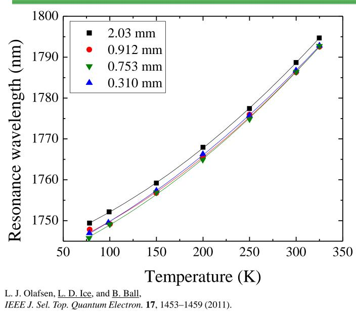
The resonance pump wavelength of OPIC lasers is consistently observed to demonstrate quadratic temperature dependence for a variety of cavity lengths and locations on the epitaxial wafer.
