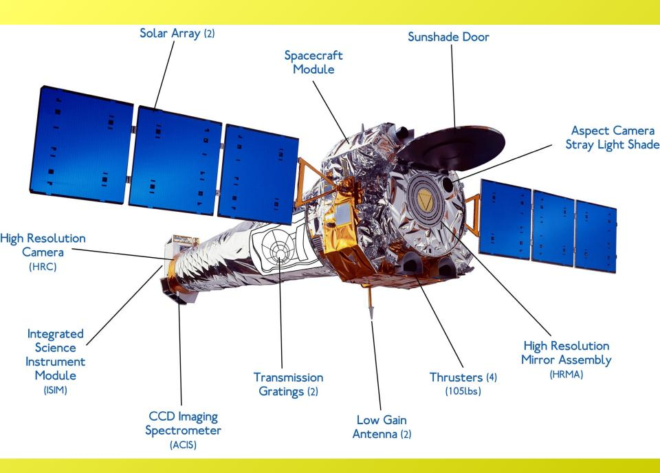
Chandra Gratings: High-Energy **Transmission Grating (HETG)** Grating Resolutions: (1 Å = 0.1 nm)-HEG: 0.012 Å = 0.0012 nm-MEG: 0.023 Å = 0.0023 nm• Energy Resolutions  $E/\triangle E$ : -HEG (at 6 keV): ~1000
