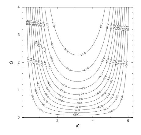
Figure 3.6: Amplitude error contours for isothermal SPH with artificial viscosity on the  $\kappa - \alpha$  plane.  $b_{SPH,AV}$  is always negative, so the amplitude of the initial perturbation decays with time. The contours show the values at the time, t = 1, i.e. just after one period of the wave. The amplitude error depends very weakly on  $\alpha$  in the stable region. This means that provided  $\alpha$  is set in the stable region, the value of  $\alpha$  is not very critical.
