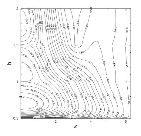
Figure 3.7: Phase error contours for isothermal GPH. At all wavelengths,  $\omega_{GPH}^2$  is positive, and the general trend is very similar to the case of SPH without artificial viscosity.
