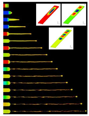
**Figure 2.** Inter-disciplinary simulation of piezoelectric inkjet formation. Time interval is 6% of firing cycle.
