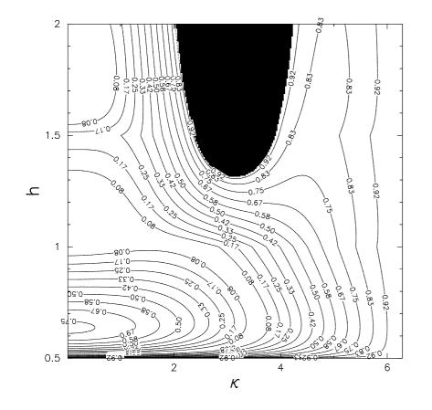
**Figure 3.5:** Phase error contours for isothermal SPH with artificial viscosity.  $\alpha$  is set to 1. The region filled by black in the upper-middle area is the unstable region. In this region,  $\omega_{SPH,AV}^2$  is smaller than 0.
