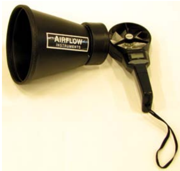
Fig. 3.19 Anemometer with volume flow hood
