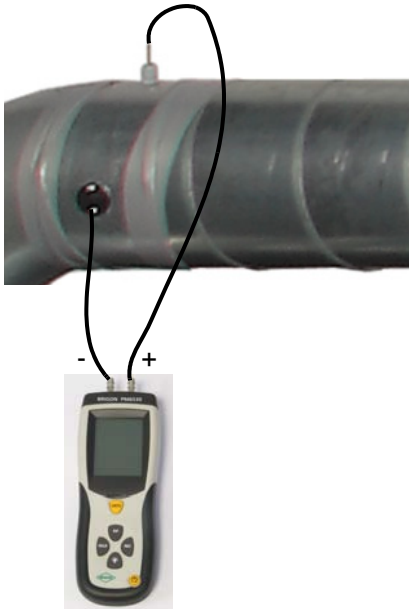
Fig. 3.23 Measuring dynamic pressure with the digital manometer
