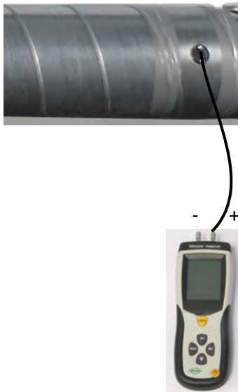
Fig. 3.21 Measuring the pressure relative to the atmospheric pressure
